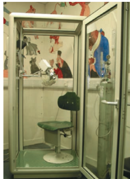
Fig. 6.4: Body plethysmograph—used to measure lung volumes
