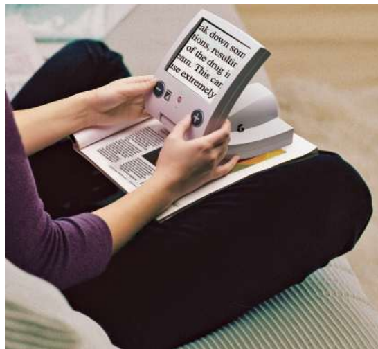
Fig. 27.38: Magnifying aids for reading with visual impairment (Traveler + portable video magnifier, available from Optelec-www.optelec.com)
