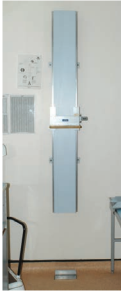
Fig. 2.3: Wall mounted stadiometer for height measurement
